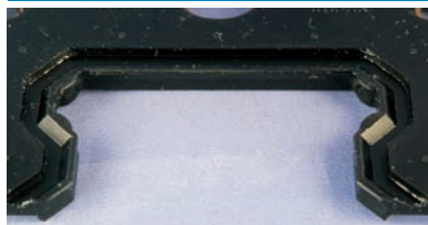
Lip has not been fractured
