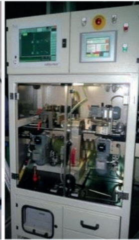
Crack detection EDDY currents
